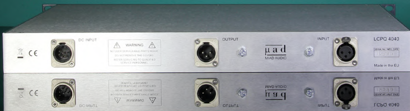
The DC input accepts a cable from the separate PSU, which can supply power to two LCPQ 4040s.
